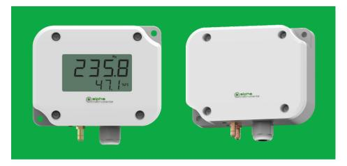
The Model 172 series are low-range differential pressure transmitters with capacitive sensors. The patented stainless steel diaphragm sensor provides excellent corrosion resistance, repeatability, and long-term stability.
